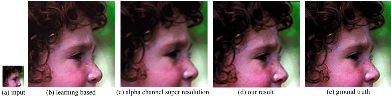
Figure 8. Super-resolution comparison (4X) of learning based method [10], alpha channel super-resolution [6], and our approach. Both large scale edges and small scale details (on the face) are recovered in our result.
