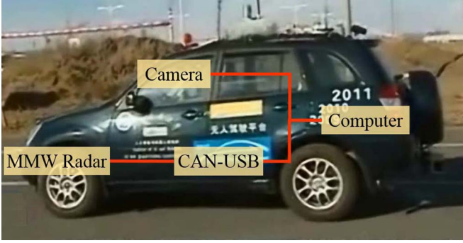
Fig. 1. The hardware platform of our “Kuaifu-II” intelligent vehicle.
