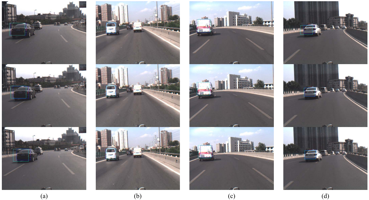
Fig. 12. Examples of vehicle tracking results. Three consecutive frames for four different kinds of vehicles are illustrated: (a) a black saloon, (b) a white minibus, (c) a truck, and (d) a white sedan.
