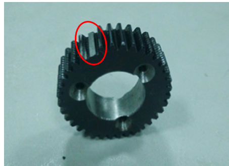
Fig. 15. Broken tooth fault of the first stage planet gear.
