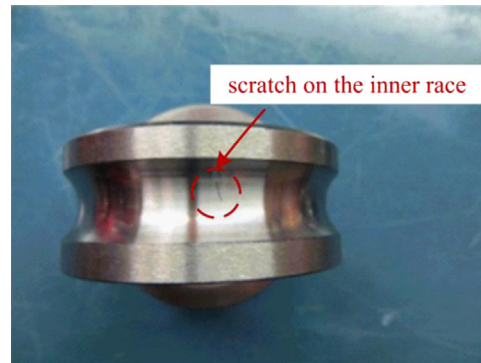
Fig. 12. The test bearing with inner race defect.
