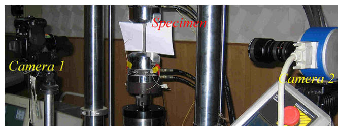
Fig. 2. The test set-up of the displacement measurement system.
