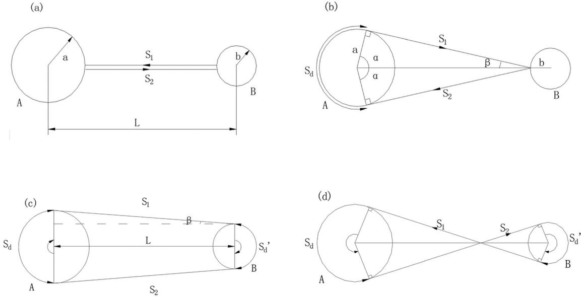
FIG. 5. External oscillation periodic paths of the first and second order scatterings of the two-cylinder system (radii  $a \neq b$ ). (a) Geometric reflected waves, total reflection between cylinders A and B; (b) diffraction by A and reflection by B; (c) diffraction by A and B; and (d) cross diffraction by A and B.
