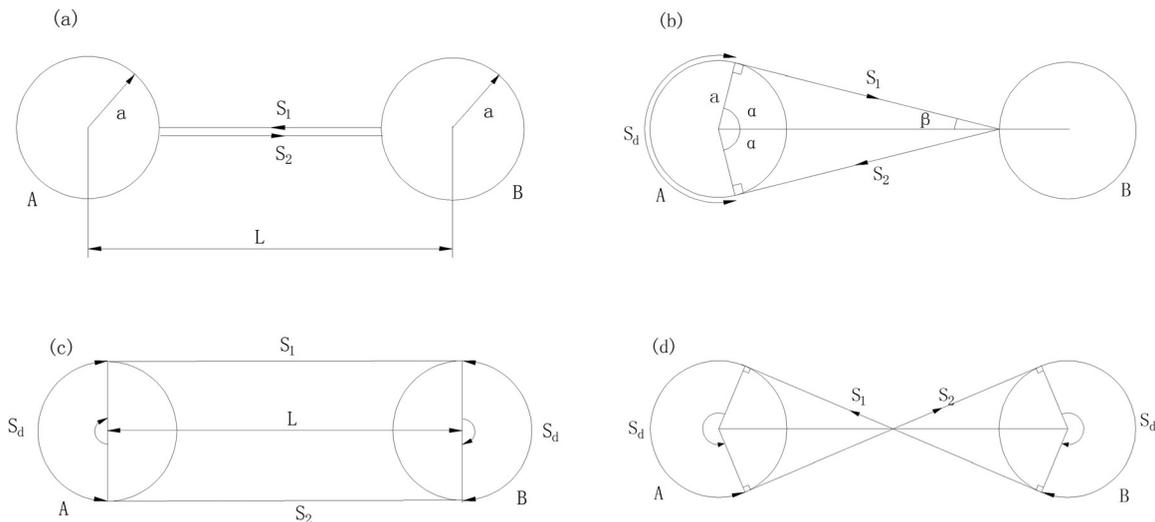
FIG. 2. External oscillation periodic paths of the first and second order scatterings of the two-cylinder system (radii  $a = b$ ). (a) Geometric reflected waves, the total reflection between cylinders A and B; (b) diffraction by A and reflection by B; (c) diffraction by A and B; and (d) cross diffraction by A and B.
