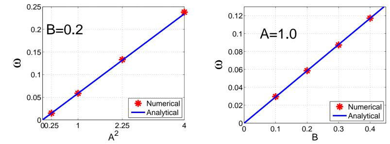
In the range of stability of the azimuthons the angular frequencies predicted by Eq. (4) coincide with those obtained from the numerical simulations (red stars).
