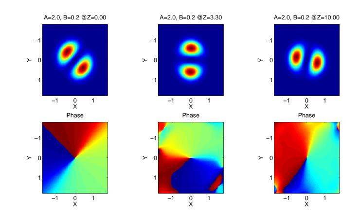
The angular momentum is changing sign periodically, because the azimuthon swings back and forth during propagation.
