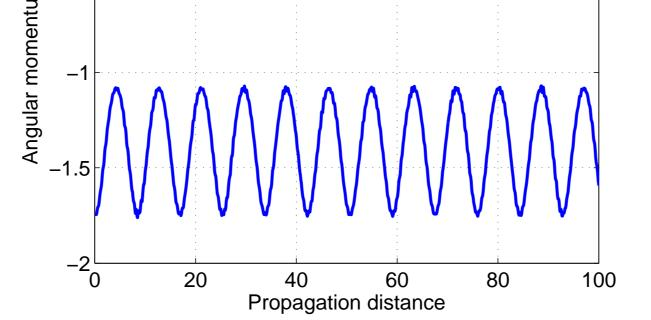
The angular momentum  $-i \iint \psi^* \partial_{\phi} \psi dX dY$  is changing periodically, because the angular frequency of the azimuthon is not constant during propagation.
