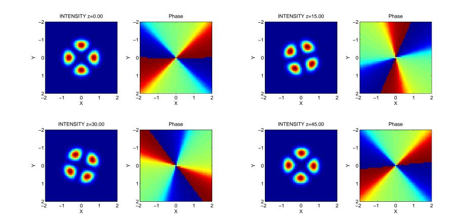
• In a square waveguide, higher-order azimuthons always swing back and forth during propagation. Here, the next pair of degenerated waveguide modes are hexapoles. The quadrupole modes are not degenerated, and propagation dynamics of a superposed state in weakly nonlinear regime is dominated by linear mode beating. The following figure shows propagation of the hexapole azimuthon with A = 1 and B = 0.2.
