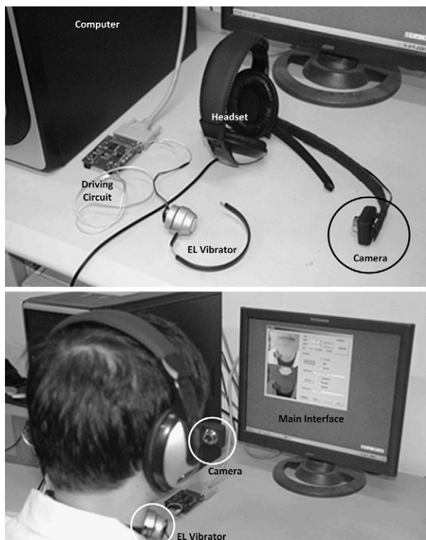
FIGURE 3. Implementation of the video-EL system. The upper image shows the composition of video-EL, and the lower image shows a subject using video-EL.
