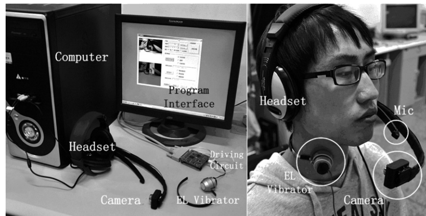
FIGURE 2. The experimental electrolarynx (ANN-EL) system, which is used by an individual for hands-free EL speech.
