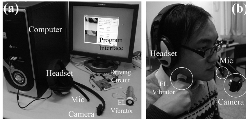
Fig. 2. The experimental electrolarynx (SGVS-EL) system. (a) Photo of system components. (b) The SGVS-EL is used by an individual.
