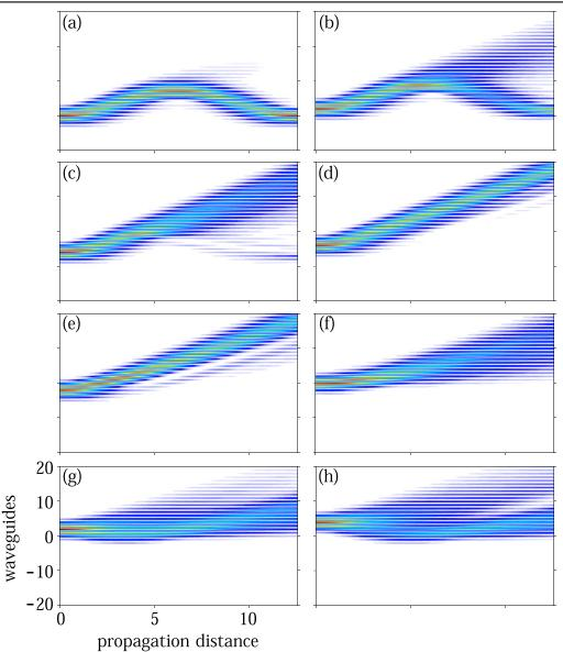
**Figure 1.** Propagation of a Gaussian light beam in a periodic waveguide array with  $\alpha = 0.5$  for  $m \le 0$  and  $\alpha = 0$  for m > 0. (a)–(h) Peaks of the incident beams are located at waveguides -10, -8, -6, -4, -2, 0, 2, and 4, respectively.
