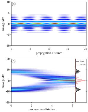
Figure 3. (a) Propagation of a Gaussian beam in a  $\Lambda$ -type modulated waveguide array with the zero waveguide excited by the beam peak. A Fermi–Pasta–Ulam recurrence-like oscillation happens during propagation. (b) Two Gaussian beams launched from positive and negative waveguide sides coalesce during propagation. The curves in the right panel depict the corresponding beam intensities at the input and output places, respectively.
