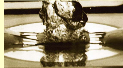
(c) q = 30.53 \text{ W/cm}^2 T_w = 81.0 \text{ }^\circ \text{C}
