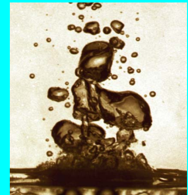
(f) q = 47.5 \text{ W/cm}^2 T_w = 75.6^\circ \text{ C}
