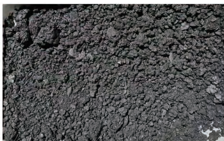
图7 1 000 °C 下石炭煤热解制得的焦样 Fig.7 Char from pyrolysis of Carboniferous coal at 1 000 °C
