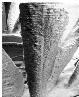
图 1 某电厂引风机叶片表面结垢积灰情况 Fig. 1 The ash deposited on induced draft fan blade of a pauler plant
