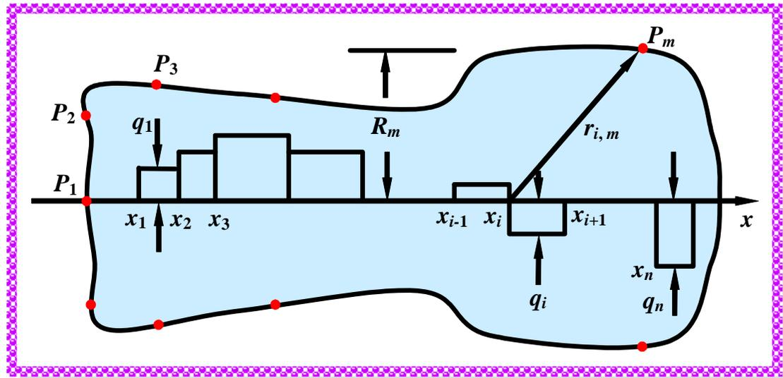
$$-\int_{x_i}^{x_{i+1}} \frac{q d\xi}{4\pi} (1 + \cos \nu) = -\frac{q_i}{4\pi} [(x_{i+1} - x_i) - (r_{i+1,m} - r_{i,m})]$$
