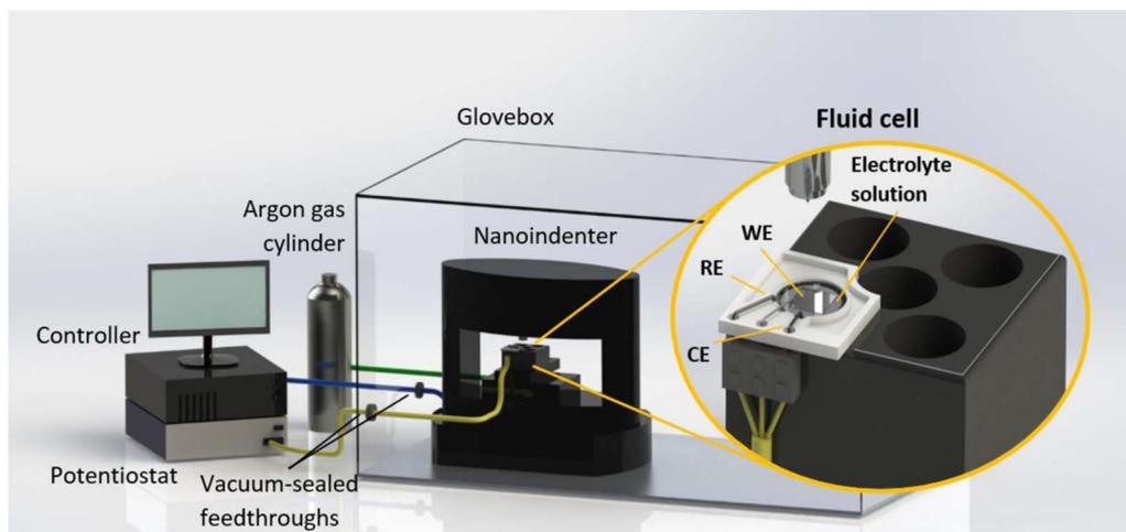
**Figure 1.** The experimental platform of operando indentation including a nanoindenter residing in an argon-filled glove box, a home-developed liquid cell, and an electrochemical station. The dynamic evolution of the mechanical properties of the working electrode (WE) is probed by nanoindentation during real-time electrochemical reactions.
