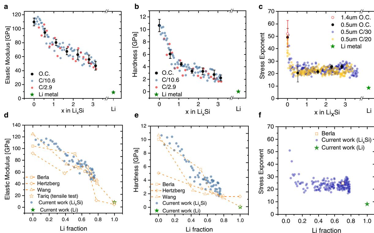
**Figure 7.** Elastic modulus, hardness, and stress exponent of Si (solid dots) measured as a function of Li concentration in open circuit (O.C.) and under various charging rates (a, b, c). The comparison of current work with the literature results by Wang et al.,<sup>58</sup> Hertzberg et al.,<sup>30</sup> Berla et al.,<sup>40</sup> and Tariq et al.<sup>57</sup> (d, e, f). Separate measurements performed on pure Li metal are included (green star).
