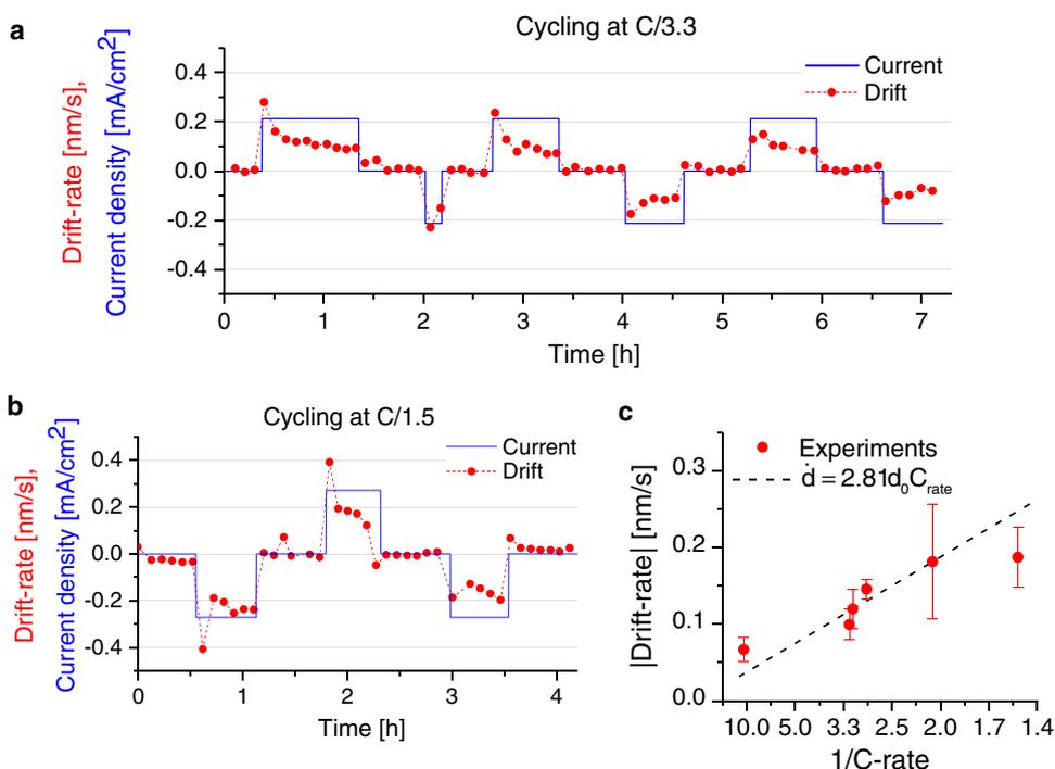
**Figure 5.** Electrochemical drift (red dots) measured during titration galvanostatic (de)lithiation (blue lines). (a) Cyclic test at C/3.3 charging rate, (b) cyclic test at C/1.5, and (c) the comparison of the drift rates with the theoretical prediction.
