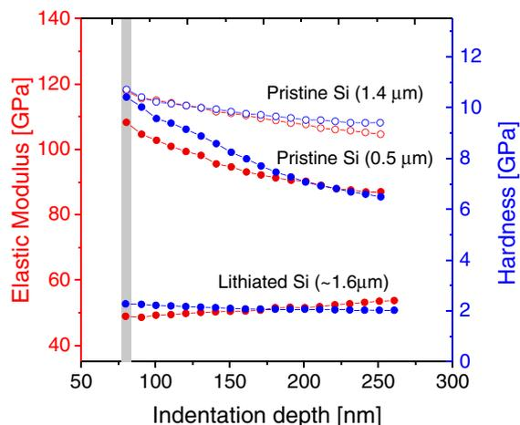
**Figure 6.** Elastic modulus and hardness as a function of the indentation depth for the Si films of 0.5  $\mu\text{m}$  ( $\sim 1.6$   $\mu\text{m}$  after lithiation) and 1.4  $\mu\text{m}$  thickness. The slopes indicate the dependence of the measurements on the film thickness and properties of the substrate. The indentation depth 80 nm (gray line) is selected as a balance between the experimental accuracy and minimization of the substrate effect.
