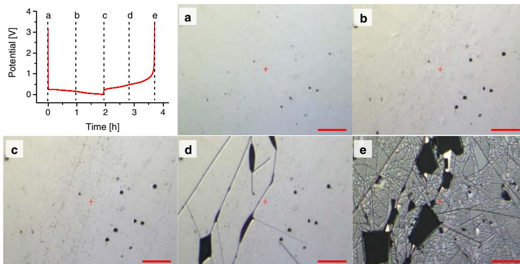
**Figure 3.** Optical images of the surface condition of a silicon thin film electrode during the first cycle at the charging rate  $C/2$  (scale bars correspond to  $100\ \mu\text{m}$ ). During lithiation (a, b, c), there is no evidence of mechanical failure and the surface is adequate for indentation tests. During delithiation (d, e), the thin film is cracked and delaminated.
