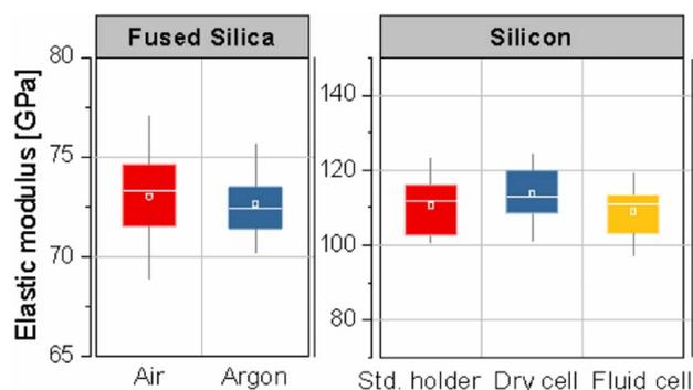
**Figure 2.** Control experiments performed on fused silica and Si thin film show that indentation tests are not affected by the argon atmosphere, customized holder (dry cell), or the liquid electrolyte environment (fluid cell).
