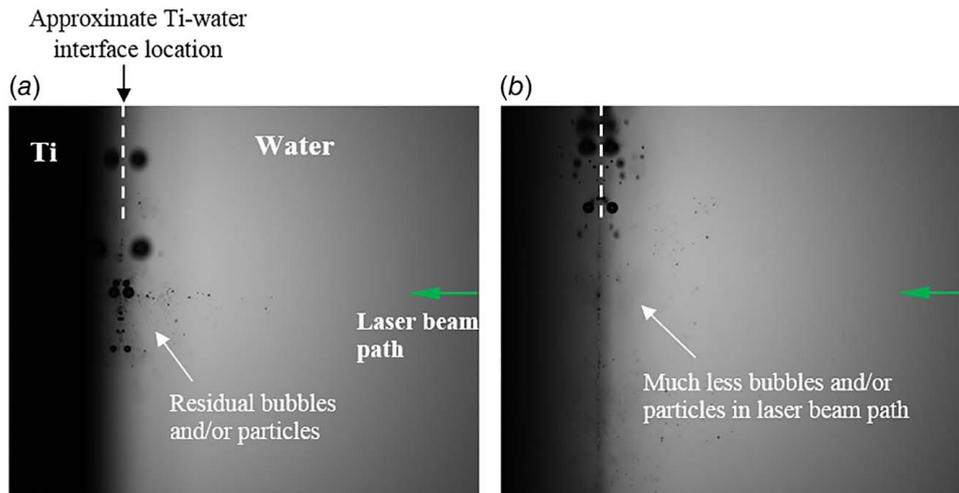
**Fig. 7** Shadowgraph images taken at  $\sim 1$  ms after 50 prior laser pulses are fired to a stationary titanium workpiece at 1 kHz pulse repetition rate for: (a) laser ablation in water without ultrasound and (b) HIFU-based UWLM (using  $100 \mu\text{s}$ -duration and 0.4 V-magnitude driving sine-wave pulses from the function generator for the HIFU transducer). Images are taken from the authors' previous paper [22], where more details can be found [22].
