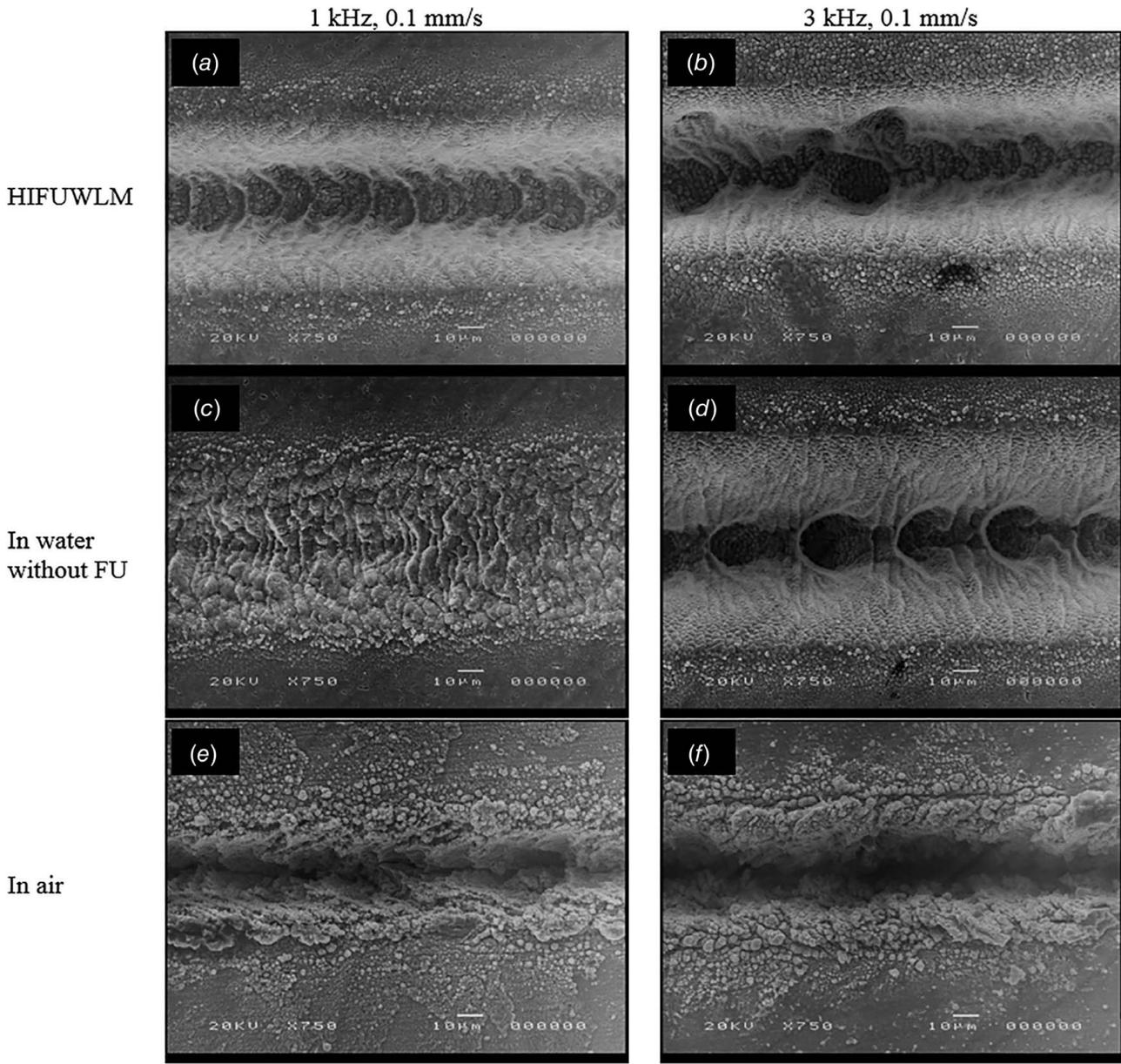
**Fig. 3 SEM images for surface grooves produced on titanium workpieces through (a and b) HIFU-based UWLM, (c and d) laser ablation in water without ultrasound, and (e and f) laser ablation in air (workpiece feed rate: 0.1 mm/s; laser pulse repetition rate: 1 kHz for the left column and 3 kHz for the right column)**
