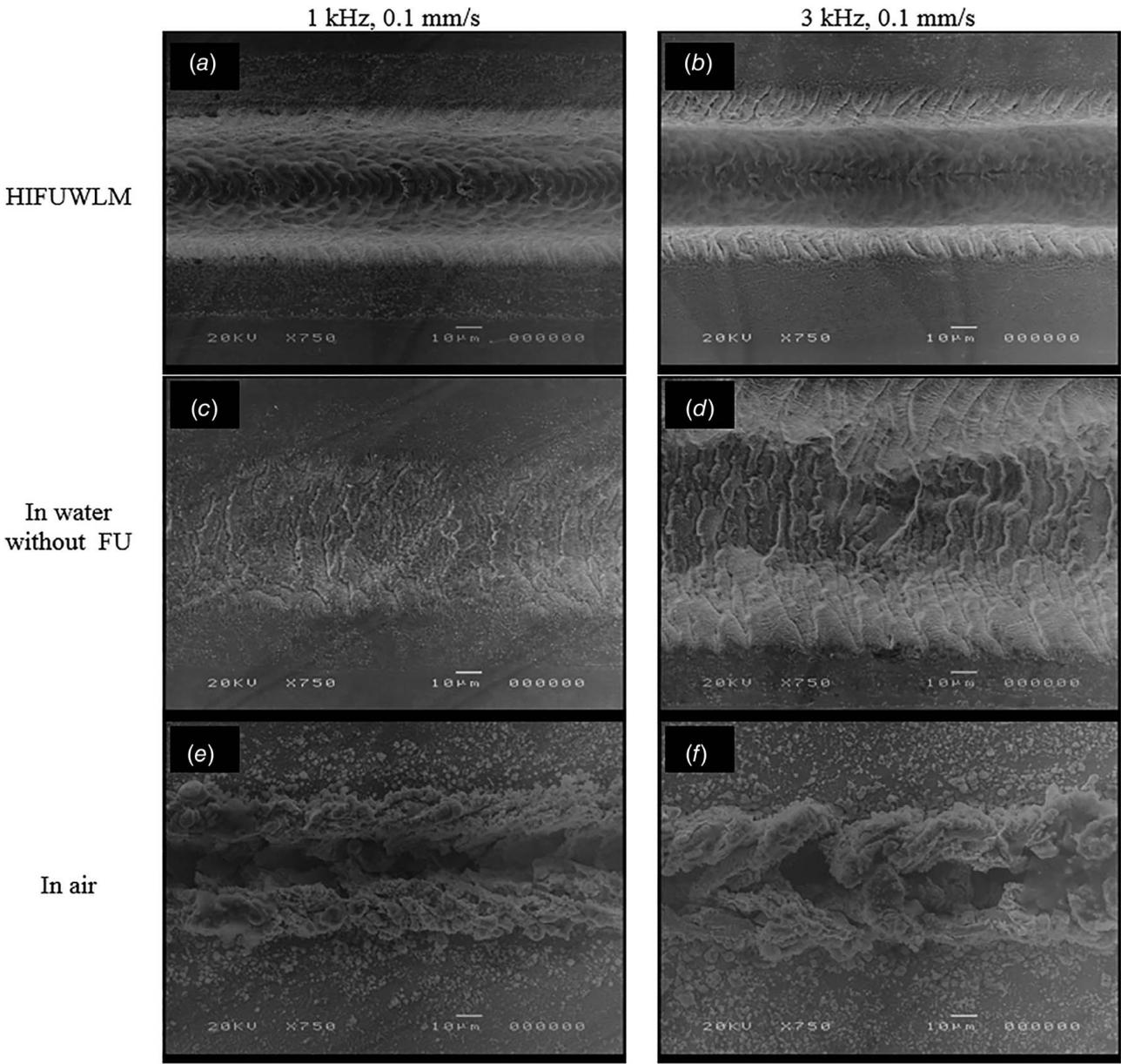
**Fig. 2** SEM images for surface grooves produced on 304 stainless steel workpieces through (a and b) HIFU-based UWLM, (c and d) laser ablation in water without ultrasound, and (e and f) laser ablation in air (workpiece feed rate: 0.1 mm/s; laser pulse repetition rate: 1 kHz for the left column and 3 kHz for the right column; HIFUWLM: HIFU-based UWLM; FU: focused ultrasound)
