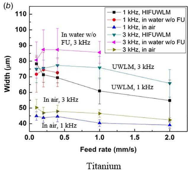
**Fig. 6** The produced groove width versus workpiece feed rate for (a) 304 stainless steel and (b) titanium workpieces under different laser pulse repetition rates of 1 kHz and 3 kHz
