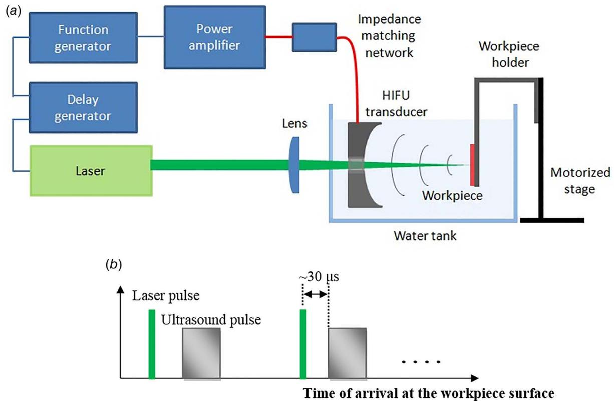
**Fig. 1** Schematic diagram of (a) the setup in this study for the grooving process using HIFU-based UWLM and (b) the relative timing of each laser and ultrasound pulse (not drawn to scale and not necessarily reflecting the exact actual sizes, shapes, or other details; not all components are shown)
