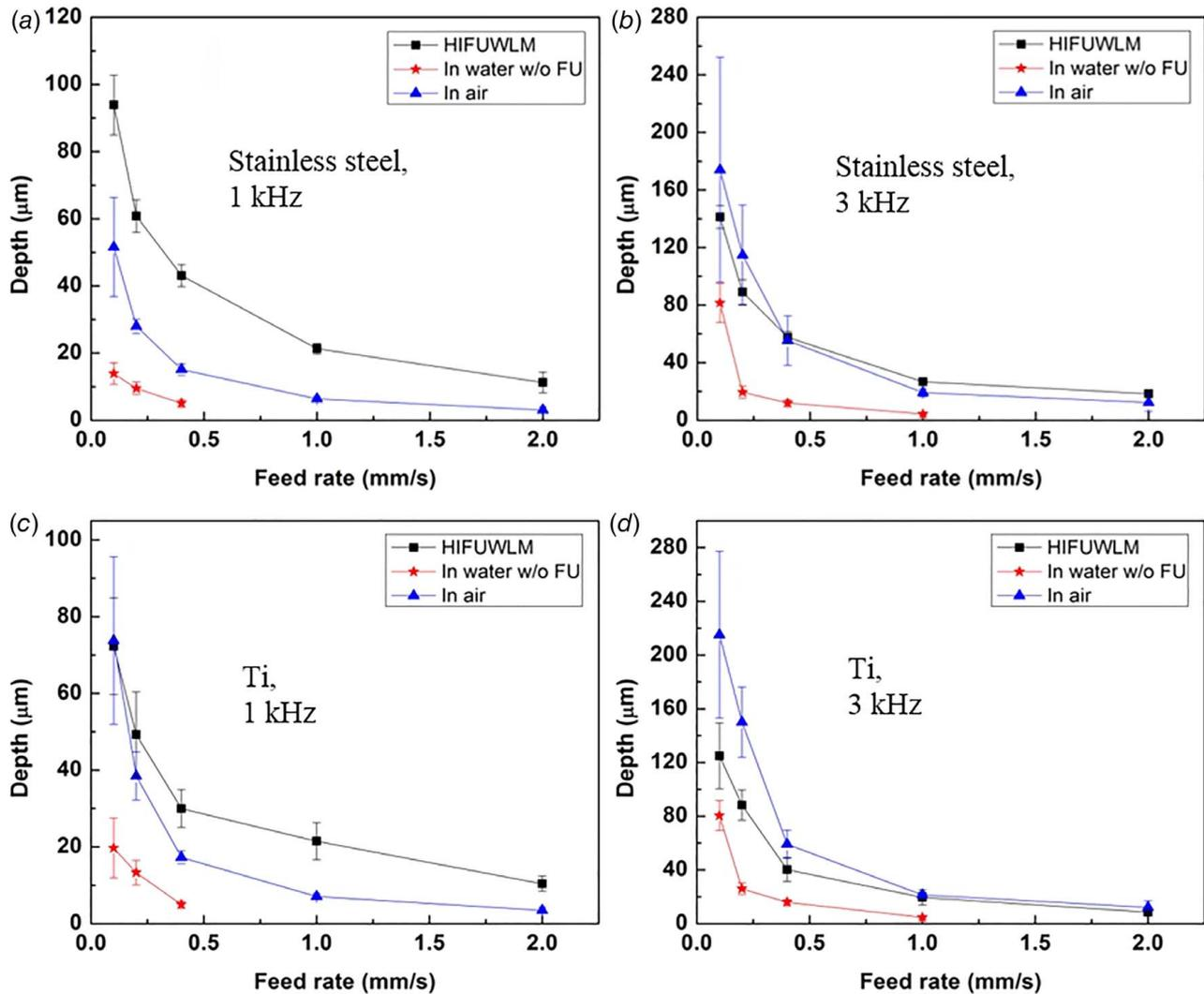
**Fig. 5** The produced groove depth versus workpiece feed rate for (a and b) 304 stainless steel and (c and d) titanium workpieces (laser pulse repetition rate: 1 kHz for the left column and 3 kHz for the right column)
