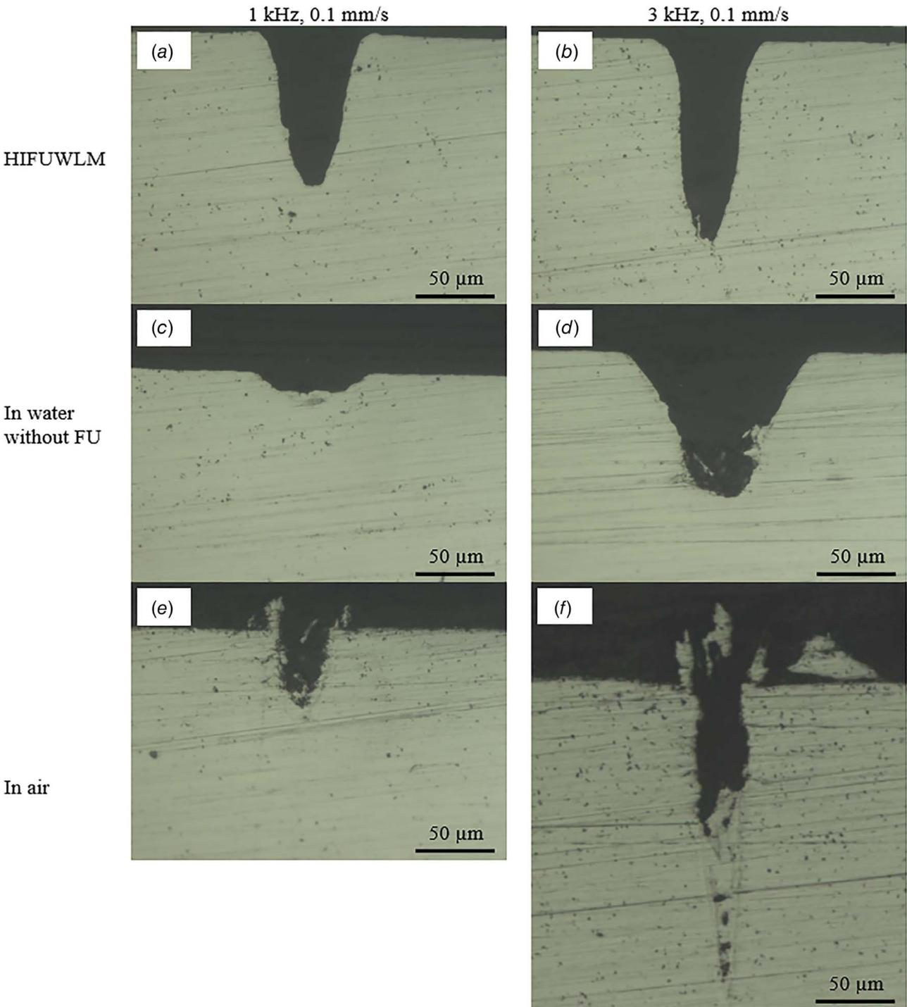
**Fig. 4** Optical microscopic images for cross sections of grooves produced in 304 stainless steel workpieces through (a and b) HIFU-based UWLM, (c and d) laser ablation in water without ultrasound, and (e and f) laser ablation in air (workpiece feed rate: 0.1 mm/s; laser pulse repetition rate: 1 kHz for the left column and 3 kHz for the right column)
