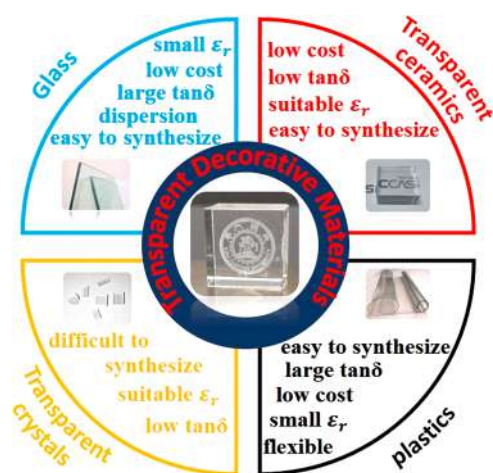
Figure 1. Schematic diagram of the performance characteristics with different transparent decorative materials.
