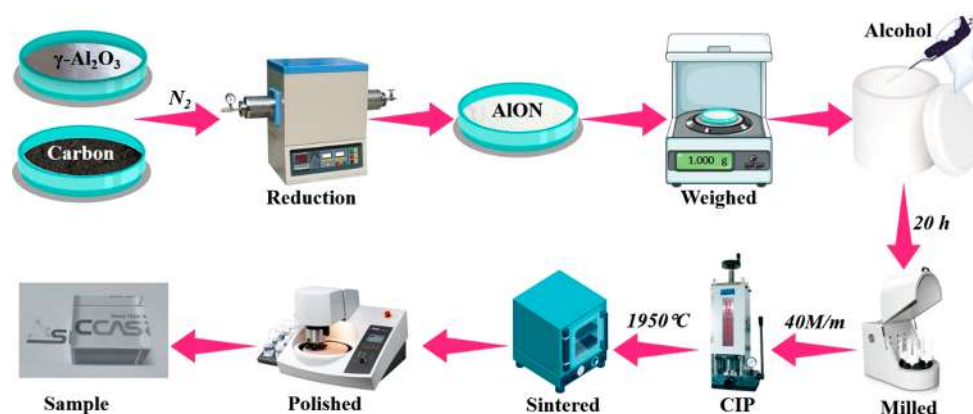
Figure 2. Schematic diagram of the experimental synthesis strategy of the AlON transparent ceramic sample.
