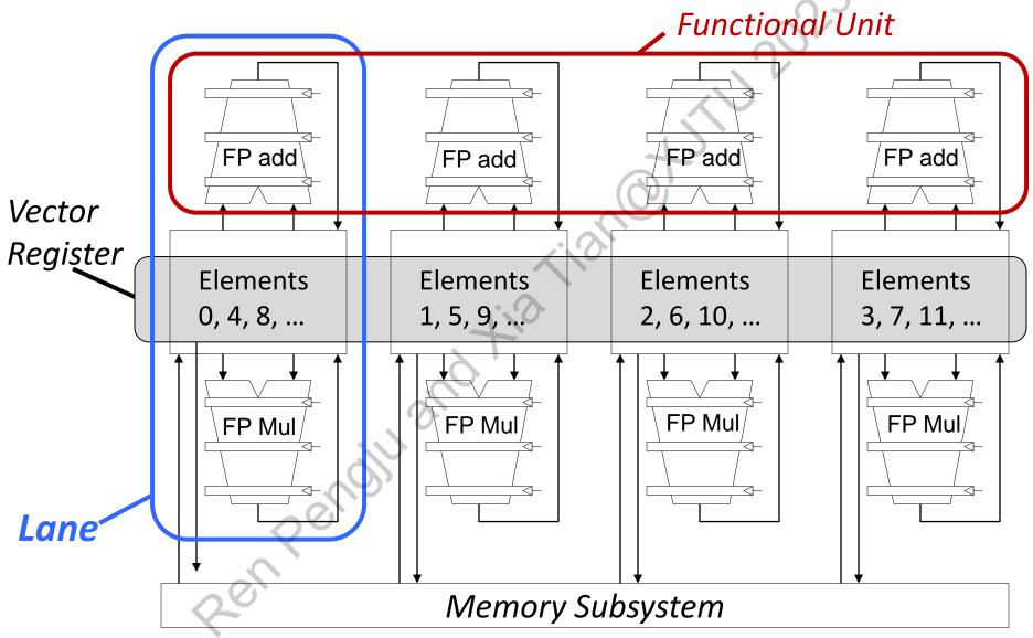
The same element position in the input and output registers is referred to as a lane.
