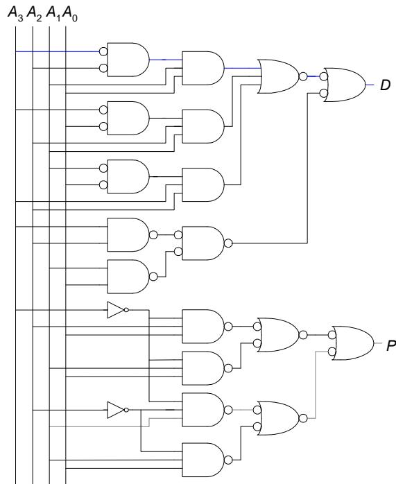
$$\begin{aligned} t_{pd} &= t_{pd\_NOR2} + t_{pd\_AND3} + t_{pd\_NOR3} + t_{pd\_NAND2} \\ &= [30 + 40 + 45 + 20] \text{ ps} \\ &= \mathbf{135 \text{ ps}} \end{aligned}$$
