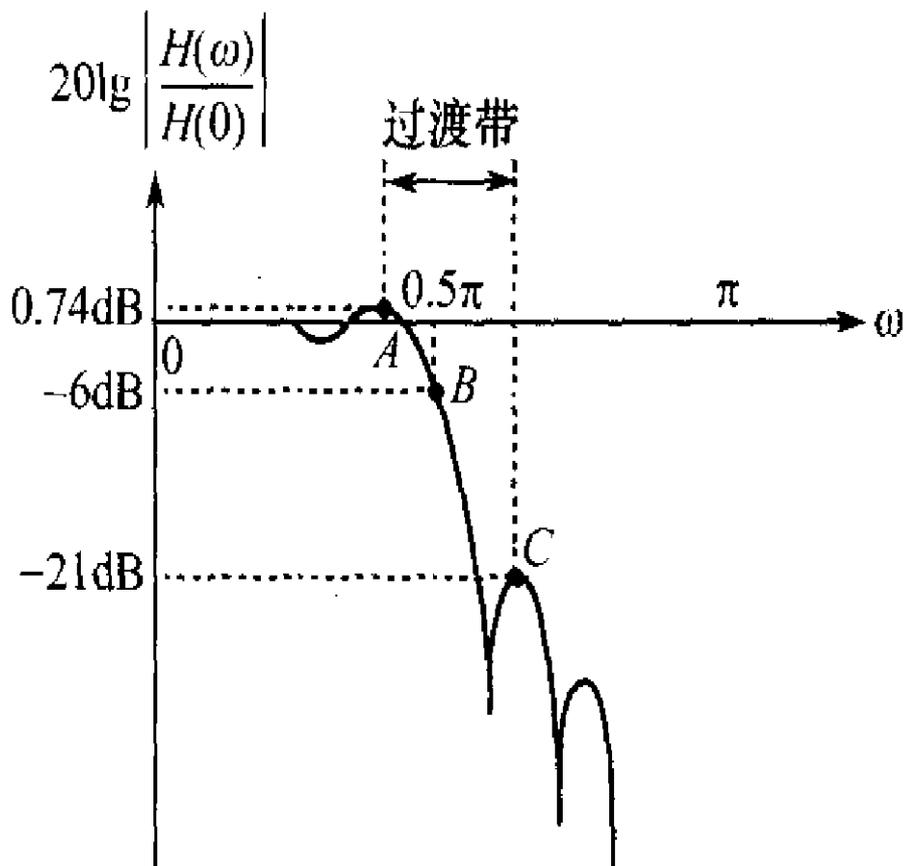
正肩峰A点:  $\omega_c - 2\pi/N = 0.5\pi - 2\pi/21$ ,  $20\lg(1.0895) = 0.74\text{dB}$
