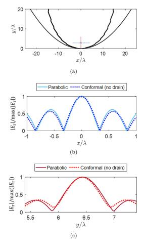
FIG. 8. Comparison between a parabolic reflector and a powerconformal metamirror without a passive drain. (a) The surface of a parabolic reflector and the conformal metamirror. (c), (d) Comparison of the normalized electric field scattered by the two structures in the *x* plane (b) and *y* plane (c) at the focal point.
