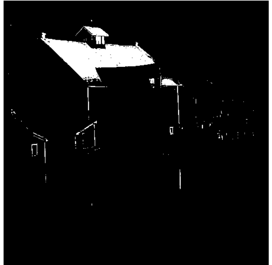
Result of thresholding with T = 210
