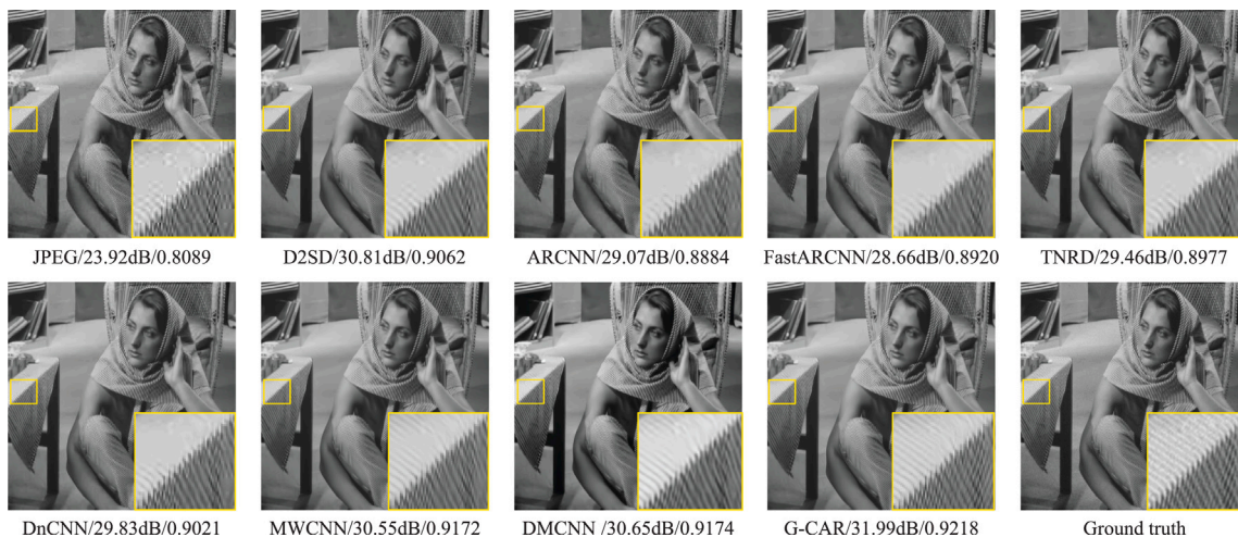
Fig. 9. Visual comparison of various deblocking methods applied on image barbara from the Classic5 dataset compressed with QF equals 20. The corresponding PSNR-B and SSIM values are presented at the bottom of each restored image.
