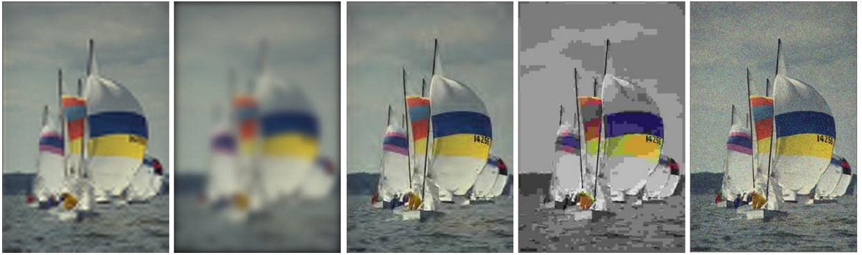
Fig. 7. Distorted versions of image sailing 2. From left to right: Fast-fading, Gaussian blur, JPEG2000 compression, JPEG compression, and white noise.
