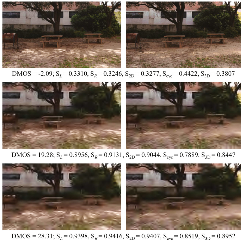
Fig. 7. Quality scores given by MUSIQUE-3D to sample distorted stereoscopic images from the LIVE 3D Phase I database.
