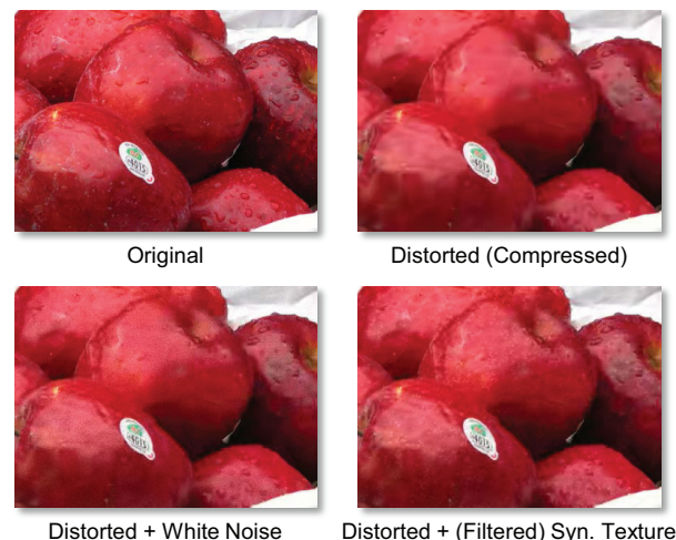
Figure 1. Demonstrative example of the potential of additive, filtered synthesized texture to improve the visual quality of a compressed image to a greater extent than additive white noise.
