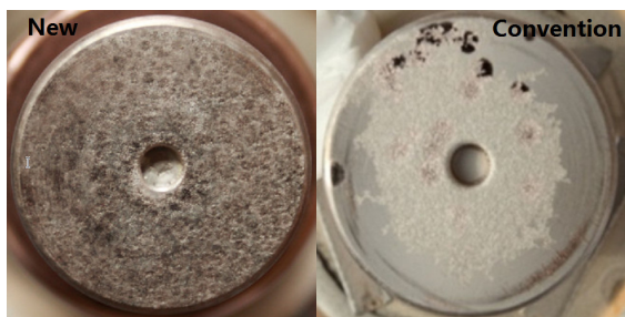
Fig. 7. The comparison of contact surfaces between new conditioning and conventional conditioning
