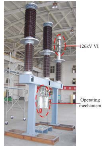
Fig. 5. 126-kV single-break VCB adopted to investigate the needed AMF strength in T100a.
