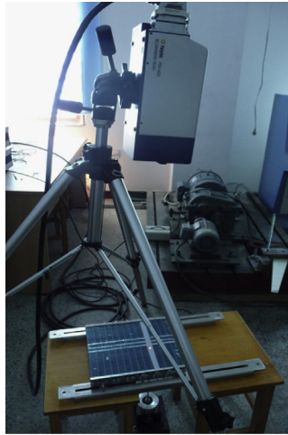
(a) Laser vibration measuring for the evaporator
